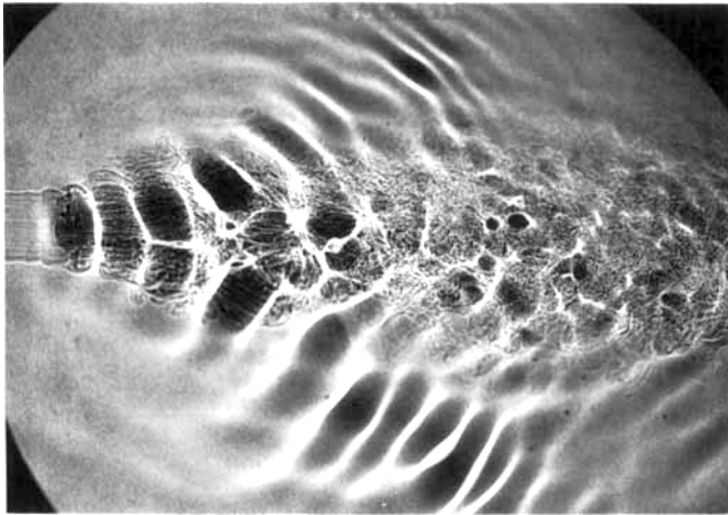
FIGURE 5. Shadowgraph image of the free-surface jet. U_e = 35 \text{ cm s}^{-1} , Reynolds number 8.9 \times 10^3 , U_e/(gh)^{\frac{1}{2}} = 0.7 , h/d = 1 . Area shown 1 < x/d < 10 .
